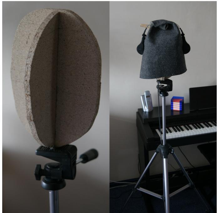
**Figure 1:** Left: frame of the dummy head used for recording indoors. Right: example set-up for indoor recordings, including the felt-covered dummy, tripod and microphones in the headband.
