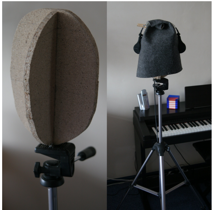
Figure 1: Left: frame of the dummy head used for recording indoors. Right: example set-up for indoor recordings, including the felt-covered dummy, tripod and microphones in the headband.
